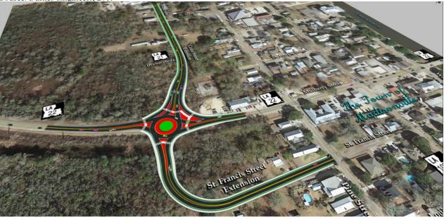
Figure 39. Vissim model overview Model depicts the proposed roundabout at LA 22 and the new LA 21, the new LA 21 and a southern connection to St. Francis Street which is part of concept 1. See draft concept one enhancements presented later in this chapter. . Source:
