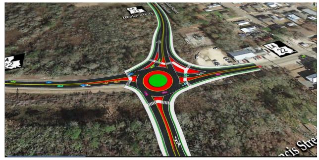
Figure 38. Vissim model of the proposed roundabout at LA 22 and the new LA 21 Source: Burkes Engineers, 2019
